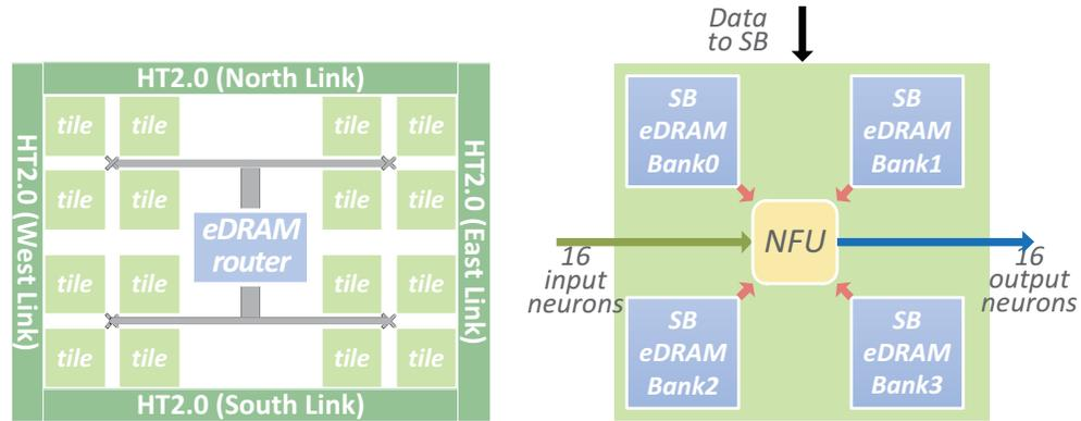
DaDiannao (Bigger Computer) uses multi-chip and EDRAM to fit larger models. Each chip is 68mm<sup>2</sup> fitting 12 Million parameters, consumes 16W
