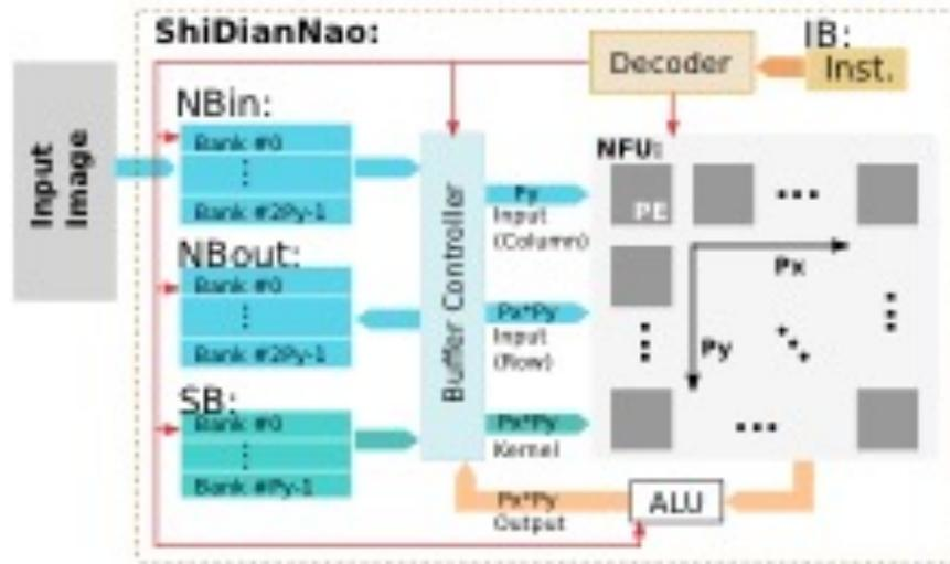
ShiDiannao (Vision Computer) It can fit small model (up-to 64K parameters) on-chip. It maps the computation on 2D PE array. The chip is 4.86 mm<sup>2</sup> and consumes 320 mW ,
