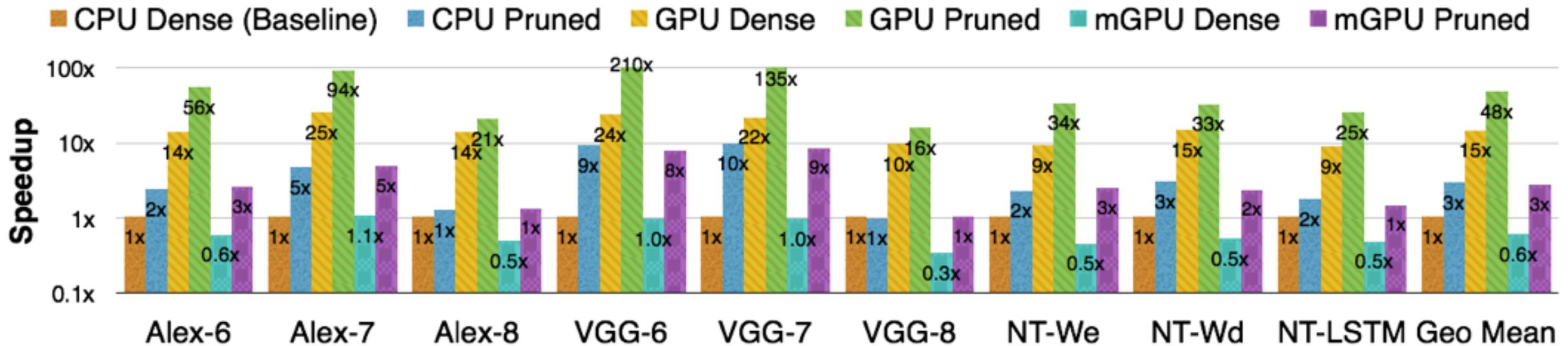
Figure 9: Compared with the original network, pruned network layer achieved  $3\times$  speedup on CPU,  $3.5\times$  on GPU and  $4.2\times$  on mobile GPU on average. Batch size = 1 targeting real time processing. Performance number normalized to CPU.
